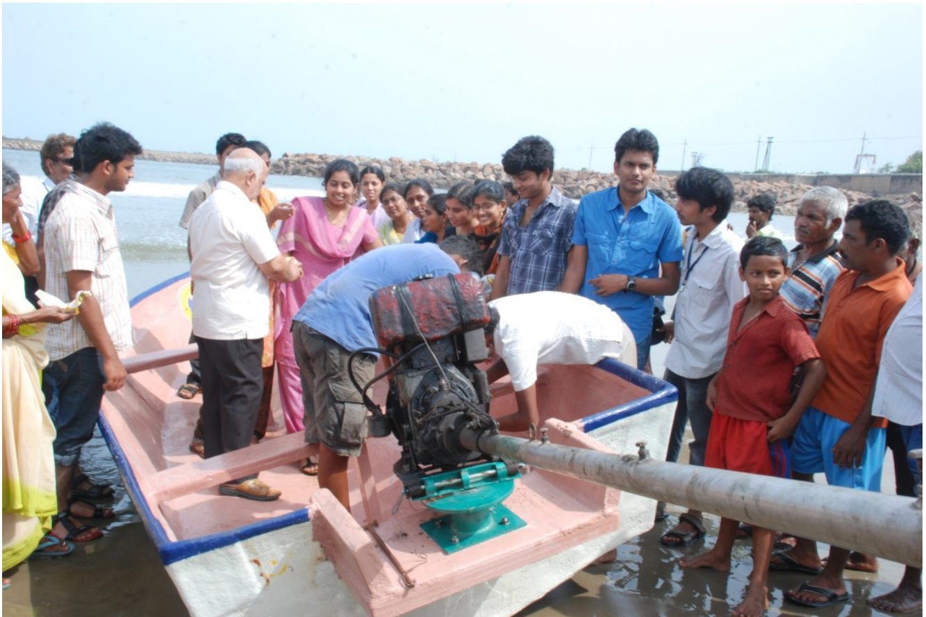
DIESEL ENGINE AND PROPELLER BEING FITTED
