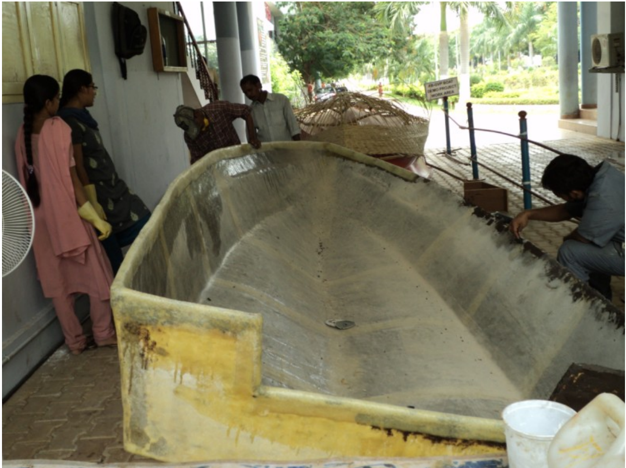
RIM OF THE DINGHY BEING CONSTRUCTED FOR EXCELLENT STRENGTH
