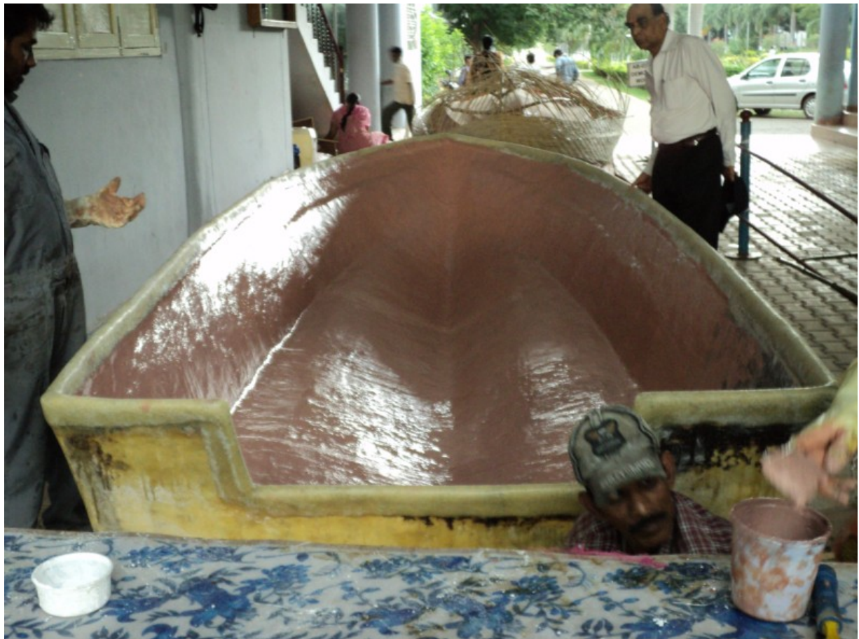
INSIDE SPECIALTY COATING BEING COMPLETED
