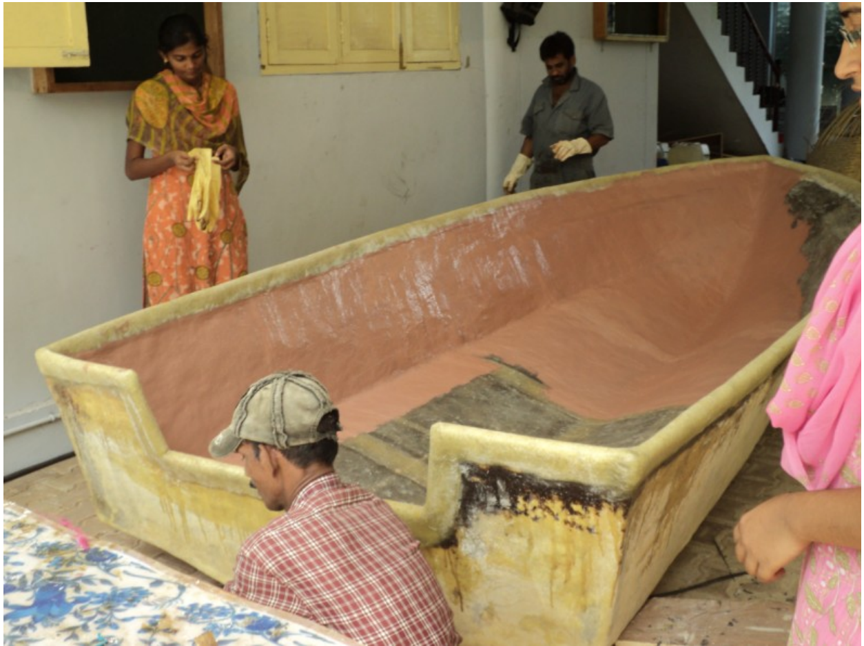
HIGH STRENGTH ULTRAVIOLET RAY RESISTANT INSIDE COATING
