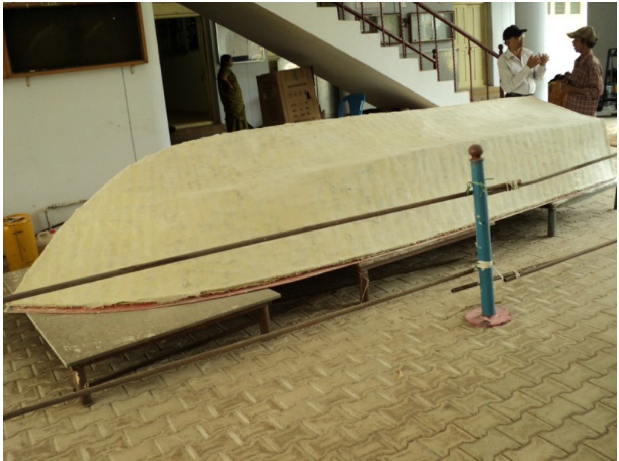
OUTER LAYERS OF GLASS FIBER + PUTTY APPLICATION COMPLETED
