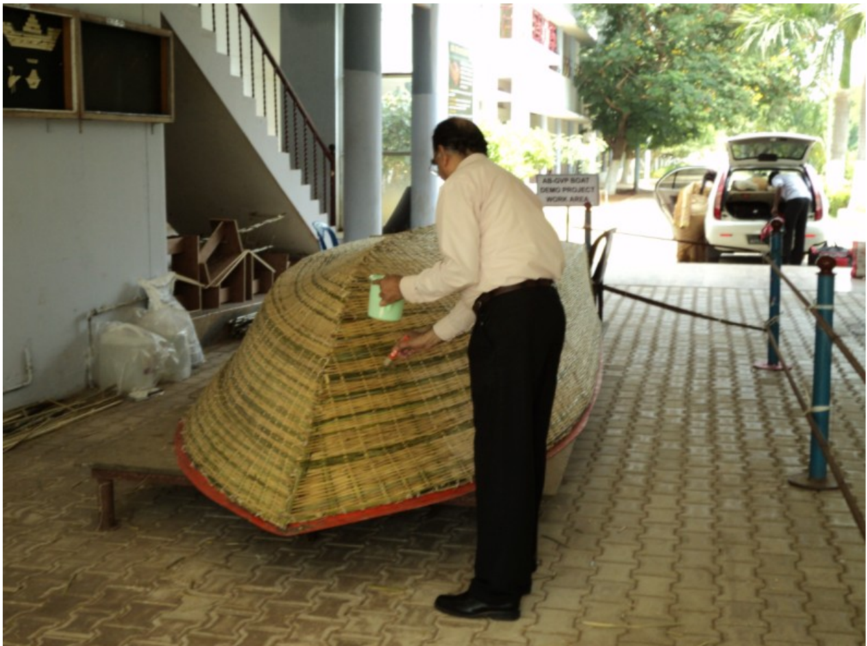
APPLYING COATING ON BAMBOO-MAT BOAT WEAVE
