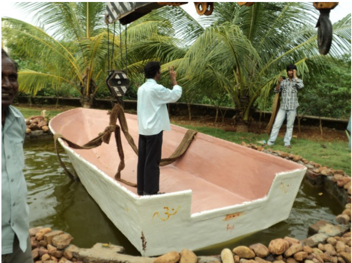
BUOYANCY TEST IN POND
