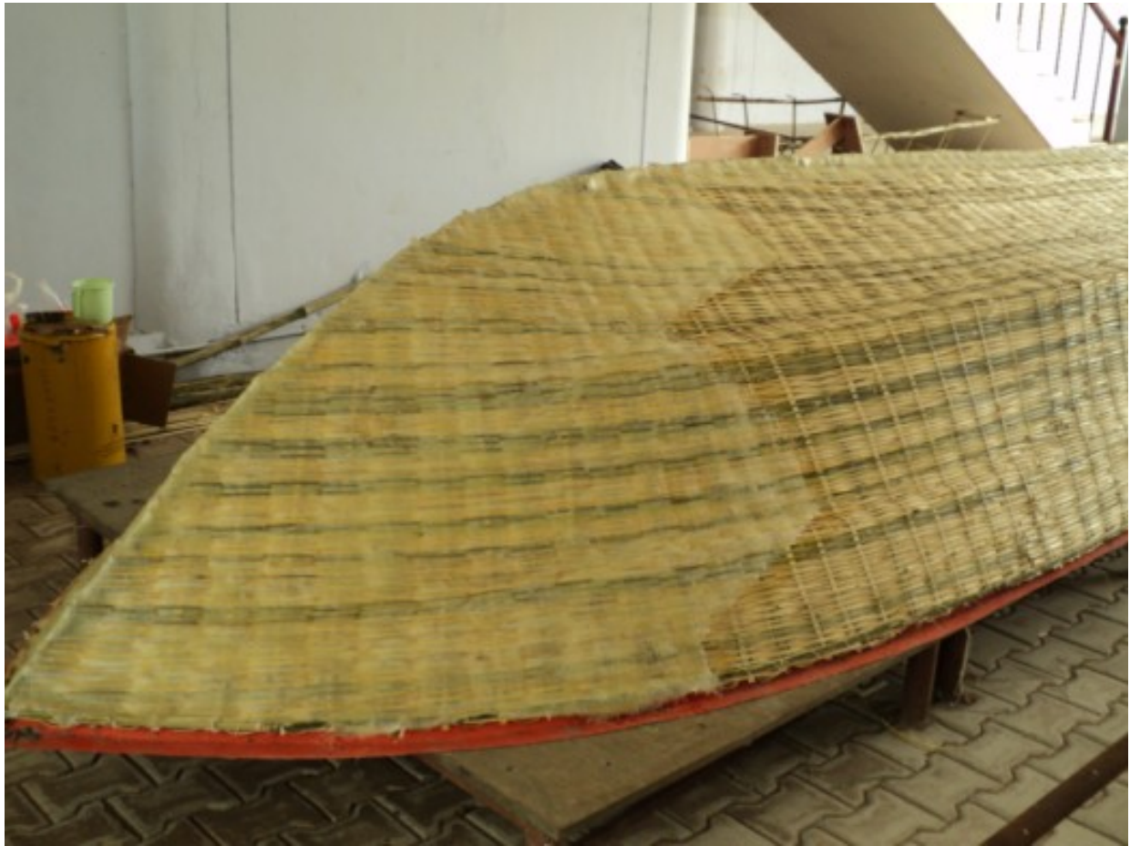
GLASS-FIBER EPOXY LAYER APPLICATION ON BAMBOO-WEAVES
